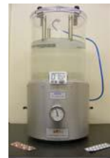
Vacuum immersion Test for Tablet Blister
